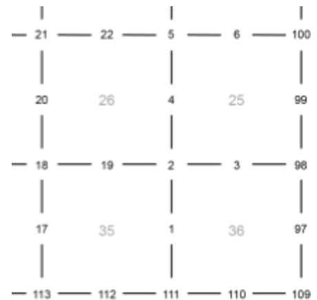
Figure 1. Township schematic showing point labels of section and quarter section corners for the sections 25, 26, 35, and 36.
